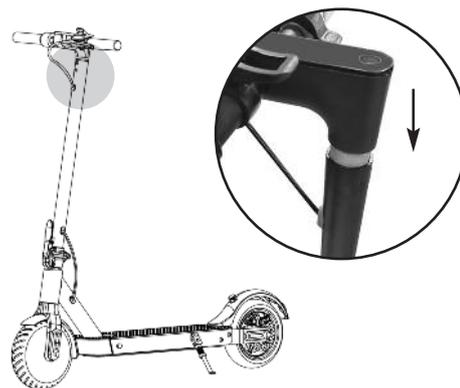
3. Secure the handlebar with the 4 screws supplied, using the M3 Allen key included.
